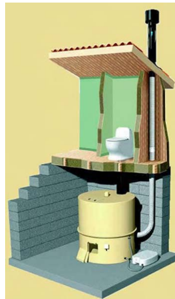
Figure 26, composting toilet system. Unlike a septic system, a composting toilet system uses the biological process of aerobic decomposition by micro-organisms, air, and heat to break down organic wastes. Source: Courtesy of U.S. Environmental Protection Agency, www.epa.gov .
