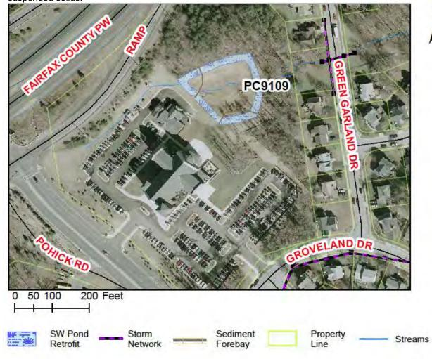
**Project Benefits:** Extending the time stormwater is detained in the pond will provide better downstream channel protection and promote particulate settlement. Installing the sediment forebays reduces debris and coarse sediment in the pond, increases infiltration, and decreases required maintenance. Below are the project's estimated pollutant removal amounts.
