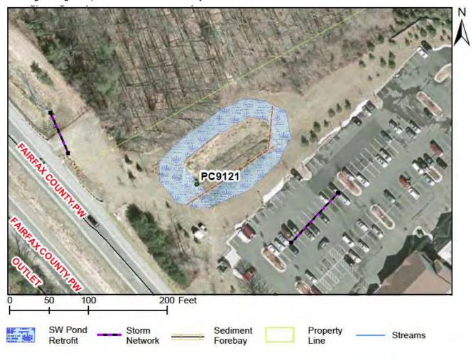
**Project Benefits:** The extended detention basin and sediment forebay will provide additional stormwater management. The sediment forebay and increased detention time will increase sediment settling and biological uptake. Enlarging the pond and adjusting the outfall structure will decrease the ponds peak discharge which will protect the downstream channel. Below are the project's estimated pollutant removal amounts.
