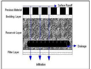
Figure 4-6: Pervious pavement section
