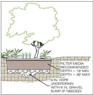
Figure 4-5: Bioretention section
