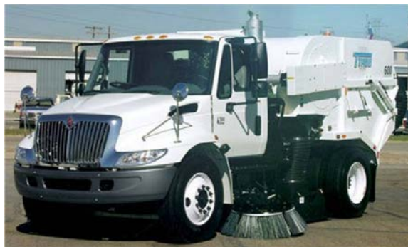
Figure 4-28: Street sweeper (Source: Tymco, Inc.)
