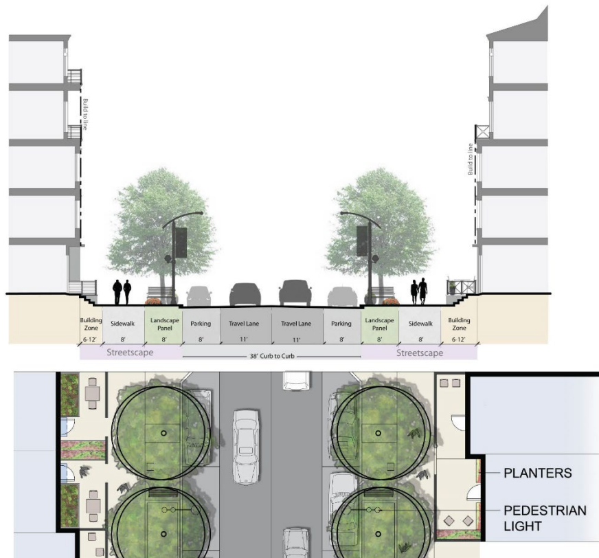
Figure 37 – Local Street Cross-section
