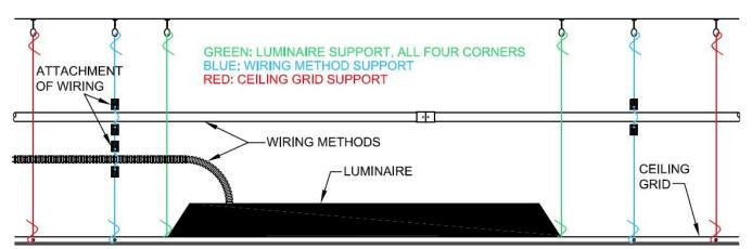
**Figure: Support of Electrical System Elements**
