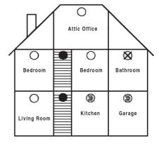
Heat Alarm lon Alarm Optical Alarm ∑ Do not fit
