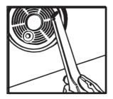
Clean the smoke alarm monthly by gently vacuuming to remove dust and cobwebs allowing proper air flow through all vents.
